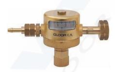
Pressure regulator with working pressure gauge, compact and robust construction. Suitable for applications where propane and oxygen are used in combination. Material of diaphragm an valve seat is NBR.
