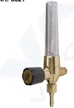
Flowmeter only, accuracy of measurement +/-10%, with shut-off valve. Calibrated to a preset inlet pressure of 4,5 bar; available for three flow rates: 0–3, 0–16 or 0–32 l/min.
