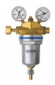
High flow rate pressure regulator (construction same as Art. 7900, but for inlet pressure up to 300 bar). With working pressure and contents gauges and integrated safety valve. Standard version with working pressure up to 10 bar. Also available with working pressure up to 20, resp. 30 bar (s.below).
