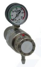
Very simple handling by setting of the desired flow-rate on the flow selector. High level of accuracy of measurement irrespective of the cylinder pressure. With integrated safety valve and gauge with indication of the cylinder pressure. The field of application is mainly in TIG, MIG, WIG and MAG welding.
