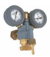
Mini pressure regulator with flow gauge, i.e. with indication I/min on secondary gauge. Integral safety valve. The flow is adjusted on the regulating screw by changing the secondary pressure and through a throttle valve in the outlet.
