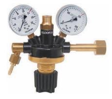
Pressure regulator with flow gauge, i.e. with indication I/min on secondary gauge. Integral safety valve. This pressure regulator is a cost effective alternative to Art.5150. With this system the flow is regulated by adjusting the secondary pressure (also via a throttle valve in the outlet).
