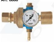
Pressure regulator with high pressure gauge (diameter 40 mm) for the indication of the cylinder content. With preset working pressure up to 8 bar (as required). Integral safety valve.
