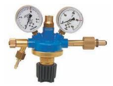
Standard pressure regulator (construction same as Art. 5100, but for inlet pressure up to 300 bar) with excellent pressure constancy. Equipped with pressure and contents gauges, integral safety valve and shut-off valve in the outlet.
