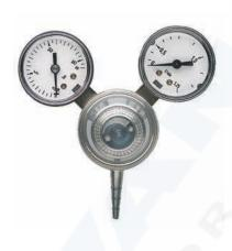
Pressure regulator with cylinder contents gauge. Flow rate with fully opened pressure adjusting screw alternatively 0.25, 0.5, 1.5 or 2.5 l/min. The pressure adjusting screw serves also as a shut-off valve. Particularly suitable for applications in which a precisely defined flow rate and secondary pressure are required.
