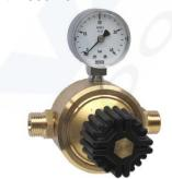
Low pressure regulator with mounted working pressure gauge and regulating screw for the adjustment of the working pressure. Diaphragm made of NBR, filter in the inlet made of sinter bronze.
