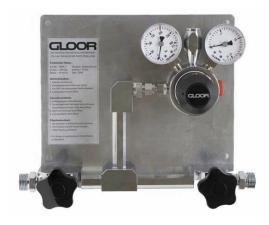
Manual change-over switching station for high purity gases with purity up to 6.0, consisting of two high pressure shut-off valves for alternate cylinder operation, main pressure regulator with safety valve, including purging valve. All parts fixed on an aluminium baseplate with specific gas identification. Option:
