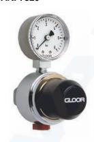
Low pressure regulator for high purity gases (6.0). Sintered filter in inlet. Pressure regulation through metal diaphragm. Working pressure fully variable as required from 0–4 or 0–10 bar.
