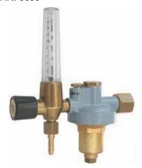
Low pressure regulator with built-on flowmeter with shut-off valve. The flowmeter design ensures a clear reading of the delivered flow rate. Accuracy of measurement of flowmeter +/-10%. Available for three flow rates (see below). Also available with ventilation valve on outlet.
