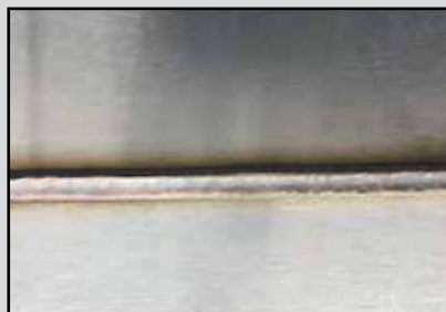
■ CrNi hoeklas PB | 2,0 mm POWER.PULS
