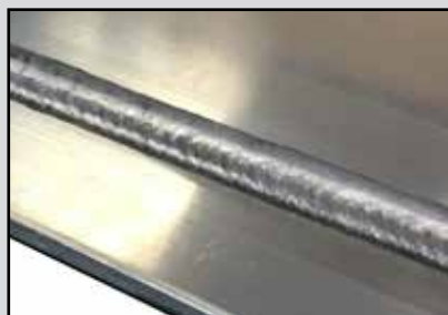
■ Aluminium hoeklas PB | 5,0 mm POWER.PULS
